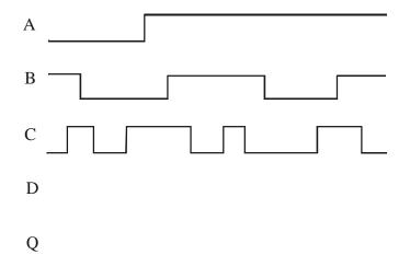
Figure 7.12 Latch Circuit Timing Diagram
