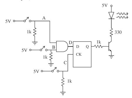
Figure 7.11 Data Latch Circuit Schematic
