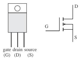
Figure 11.4 MOSFET pin-out and schematic symbol
