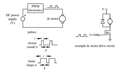
Figure 11.1 Pulse-width Modulation (PWM)
