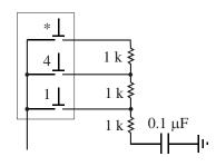
Figure 11.7 Alternative wiring for single-column keypad RC circuit
