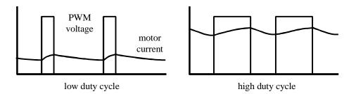
Figure 11.2 PWM voltage and motor current
