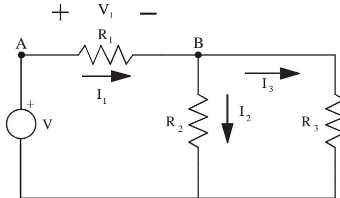
Figure 2.14 Current Divider Circuit
