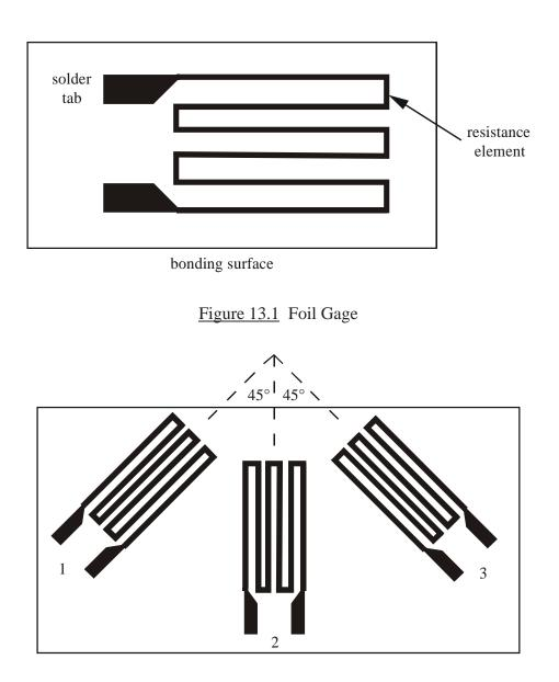
Figure 13.2 Rectangular Strain Gage Rosette
