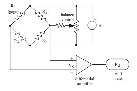
Figure 13.3 Strain Gage Conditioner Circuit
