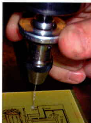
Figure 5. Drill holes for mounting components
