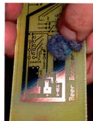
Figure 6. Use steel wool to expose the copper traces
